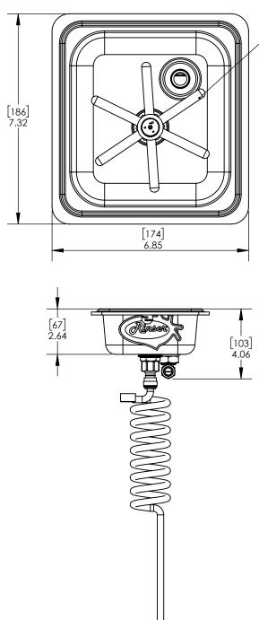
Press this Rinser Disk for functioning of Sprinkler
