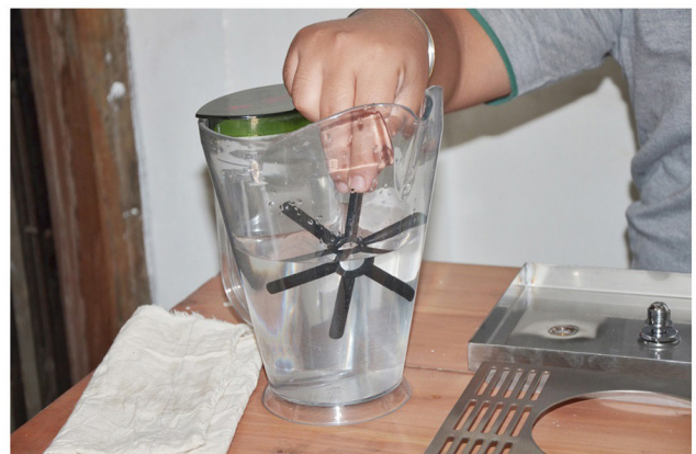
3. Remove the Rinser Disk and add the Rinser Disk to the Daily Milk Frother Cleaner solution. Allow the part to soak while cleaning the remainder of the rinser.
