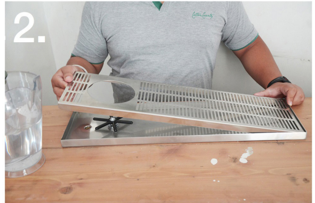
2. Remove the rinser drain tray.
