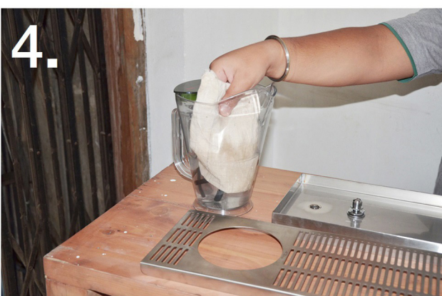
4. Dip a soft cloth into the diluted cleaning solution and use to wipe down the surfaces of the rinser. Remove soaking parts from cleaning solution and rinse.
